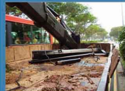
Part of the lorry crane's arm was damaged as a result of collision with a pedestrian overhead bridge at Bishan Road.
