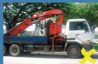
Lorry with crane partially retracted
